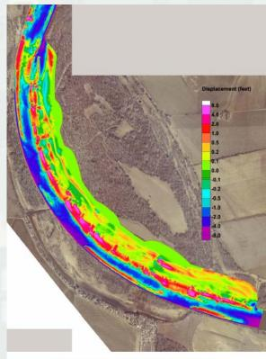
Figure 47: Bed Displacement for the 1997 Hydrograph, Option D
