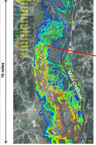
Plate 14: 1930 Reference Condition Stage Data for Total River Discharge of 32,000 cfs
