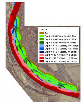
Figure 13: Depth/Velocity Zones for the August 50% Duration Flow, dmaxpx
