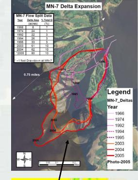
Future Without Conditions: This 7-Year Simulation of Bed Displacement in Pool 5 using ADH Matches Observed Sediment Deposition in Backwater Delta.
