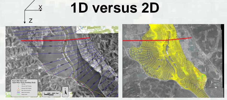
One-dimensional (1D) models simulate the change in parameters in one direction (e.g. downstream to upstream)
