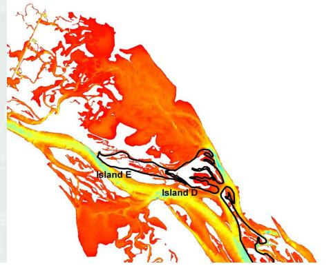
1% (100-year) Flood WSEL change due to Islands E, D, & B Island Elevations are 2 & 4 feet above Low Control Pool (LCP); Approx. Elevation 668.2 & 670.2 A Two-Dimensional Model (ADH) was used for the analysis
